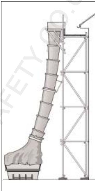
Rubbish chute and skip positioned to take waste materials
