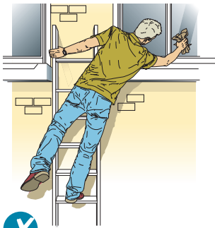
Figure 1a Incorrect - overreaching and not maintaining three points of contact
